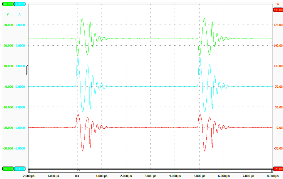
Figure 9: Time-resolved signals for input voltage (green), current (blue-green) and power (red).
