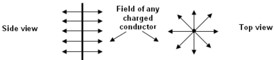
Fig.2 The electric field of any charged conductor
