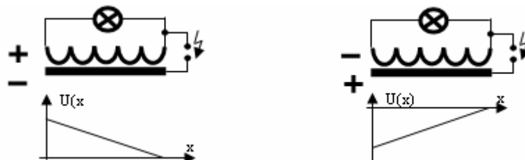
Fig.5 The manifestation of the polarity of the electro-radiant effect.
