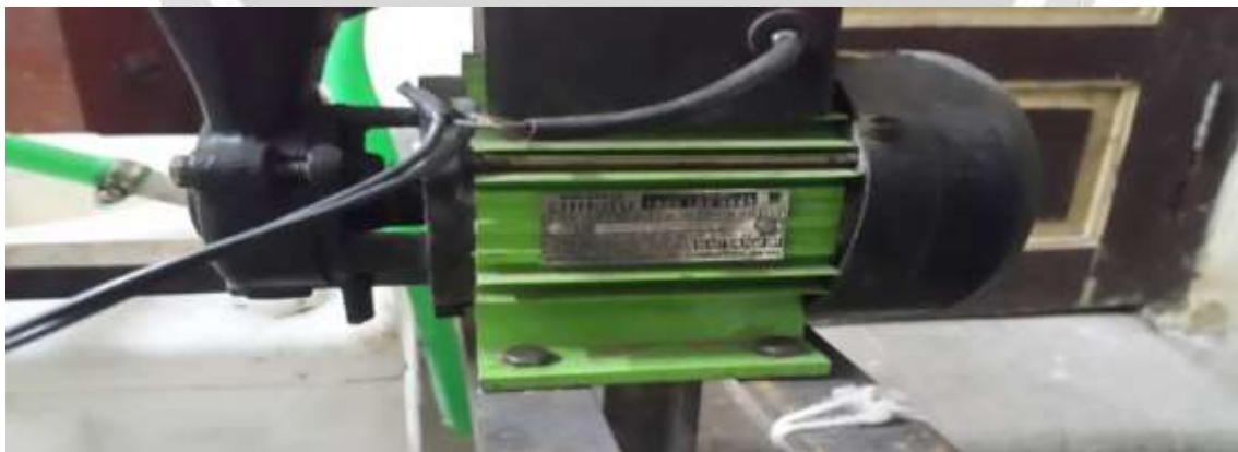
Figure 3.3 Pump and motor for operating Machine
