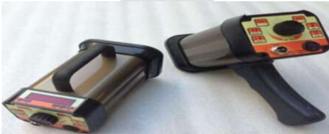
Figure 3.8 Stroboscope for measuring RPM
