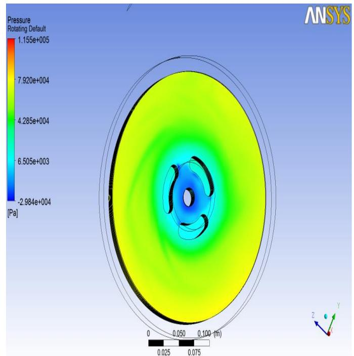
**Figure 8 Pressure gradient in rotating domain**
