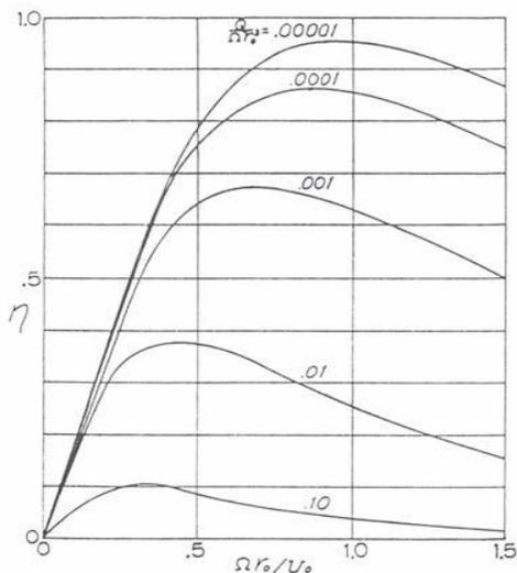
Figure 2 Typical results for maximum efficiency as a function of flow rate and parameter. Plotted for  $f=0.05$   $ro/b= 50$ [3]
