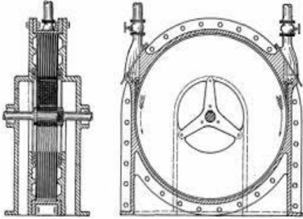
Figure 1 Original sketch of Tesla turbine [1]
