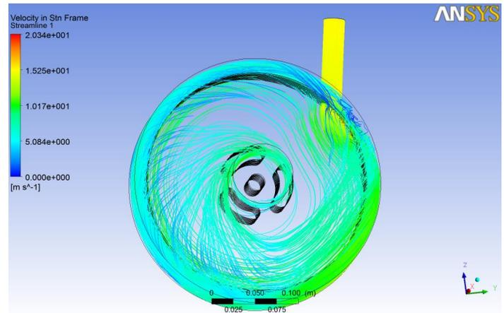
**Figure 7 Velocity streamline in stationary domain**
