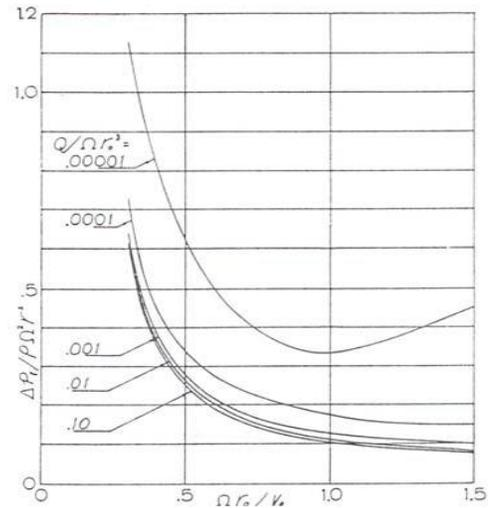
Figure 3 Typical results for pressure-change parameter as a function of flow rate and speed parameters. Plotted for  $f= 0.05$ ,  $ro/b= 50$ [3]
