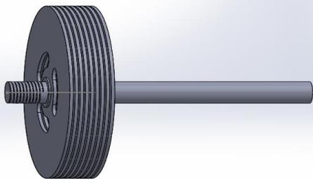
**Figure 5 Tesla turbine rotor assembly**
