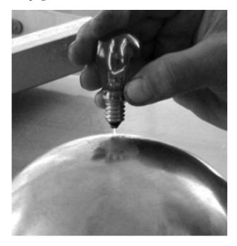
*Fig. 12 Glow of an incandescence lamp of 220V, 15Wt*
