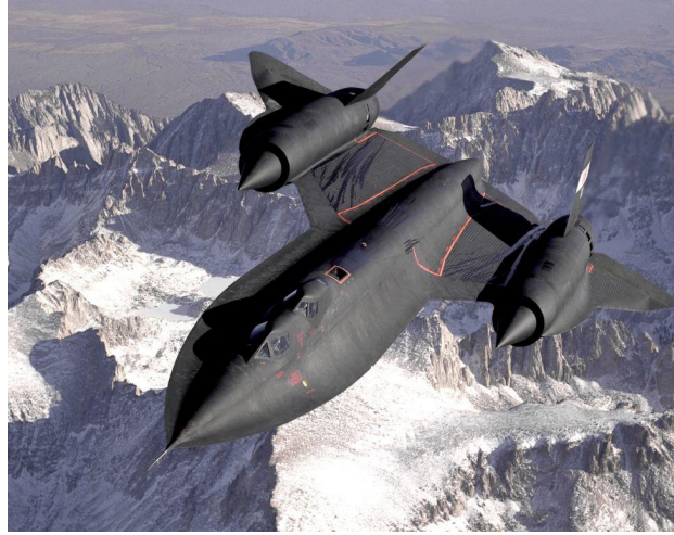
Figure 1.6: SR-71B Blackbird with translating centerbody in the intake. Taken on December 1994 from an in-flight refuelling tanker. SR-71B was the trainer version of the SR-71. Notice the dual cockpit to allow the instructor to fly the airplane. NASA Photo EC94-42883-4.
