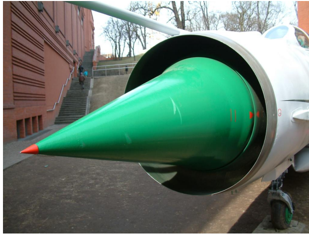
Figure 1.7: Translating nose cone intake of the Russian MiG-21 (in use from the mid 1950's). At low speeds ( M_\infty < 1.5 ) it is fully retracted; between speeds of ( 1.5 < M_\infty < 1.9 ) it is in the middle position; and at higher speeds ( M_\infty > 1.9 ) it is in the maximum forward position. Source: Wikimedia Commons.
