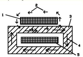
Rice. 2. The principle of excitation of a magnetic flux by electric current, which closes in addition to the closed circuit of the external field source. 1 – winding with current; 2 – magnetic field created by the current in winding 1; 3 – magnetic circuit; 4 – own magnetic flux in the magnetic circuit; 5 – secondary winding
