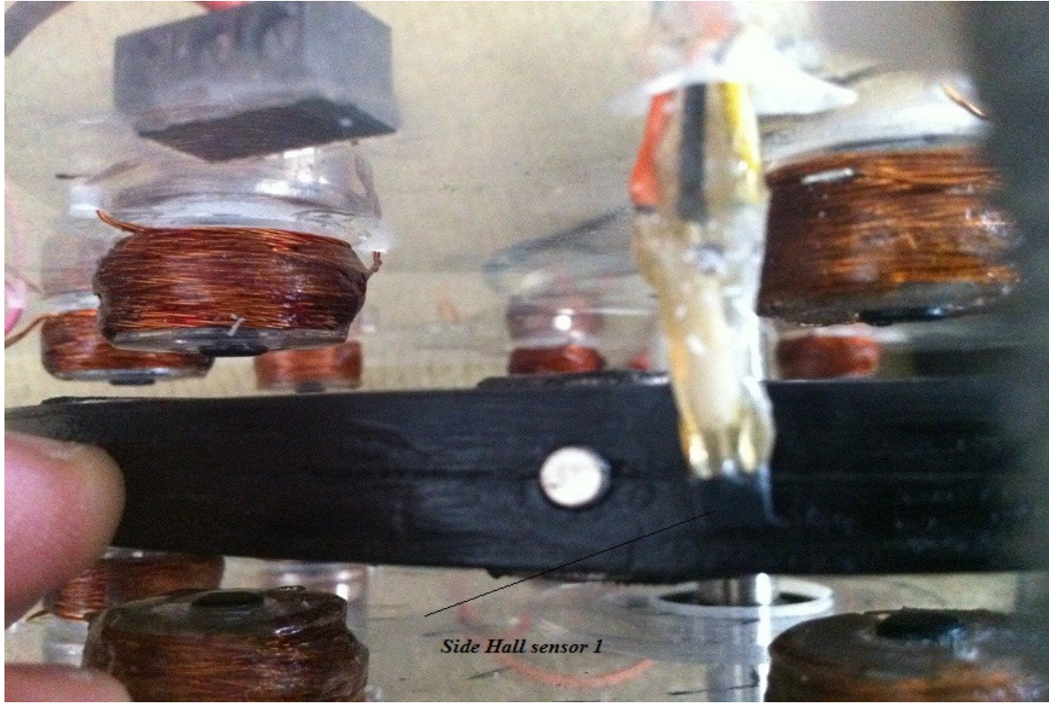
Second hall sensor uses the 8 outer magnets.
