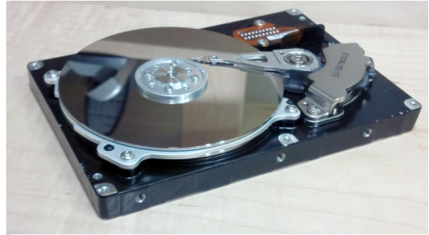
Figure 21 - A hard drive with its cover off, showing the platters.
