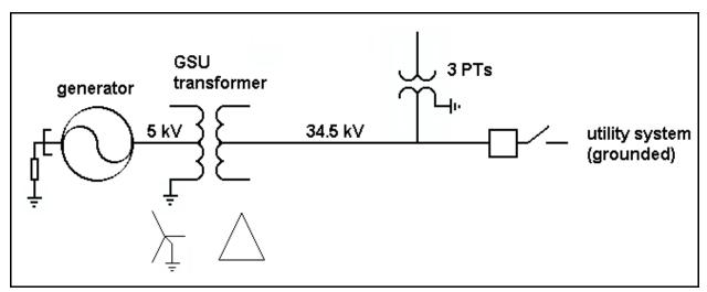
Figure 4 Typical Power System Configuration Favorable to Ferroresonance
