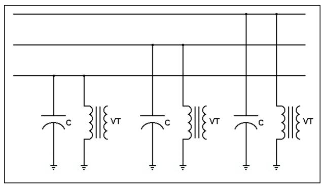
**Figure 5 Parallel Ferroresonant Circuit**
