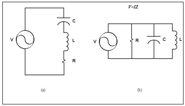
Figure 2 Series and Parallel Resonance
