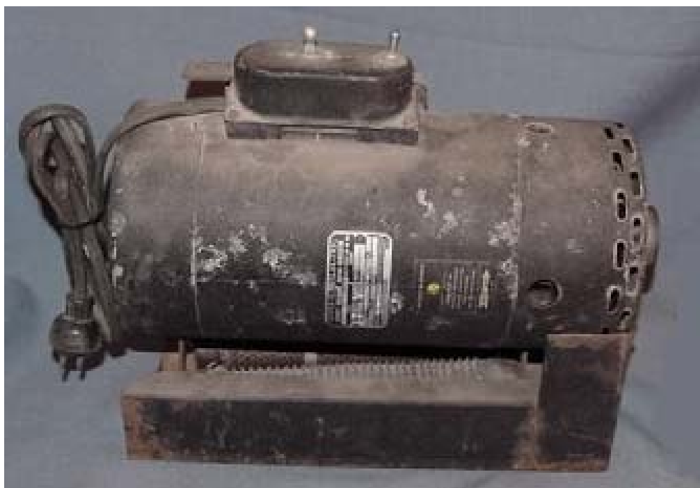
Fig 16 – A Rotating Magnetic Amplifier (Look at the Tag, General Electric)
